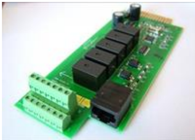
Fig. 155-4 Relay card AS400 for real time control of the UPS.
